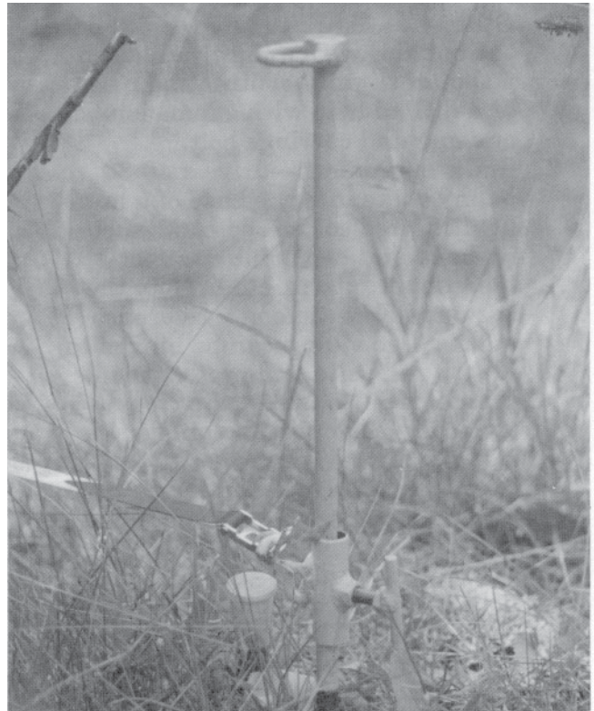
Figure 15. Rebar monument at cross-section (capped rebar on left, next to silver stake).
